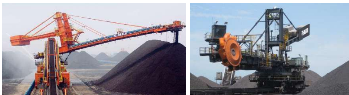
Figure 5-11: Typical mobile stacker (left) and bucket reclaimer (right)
