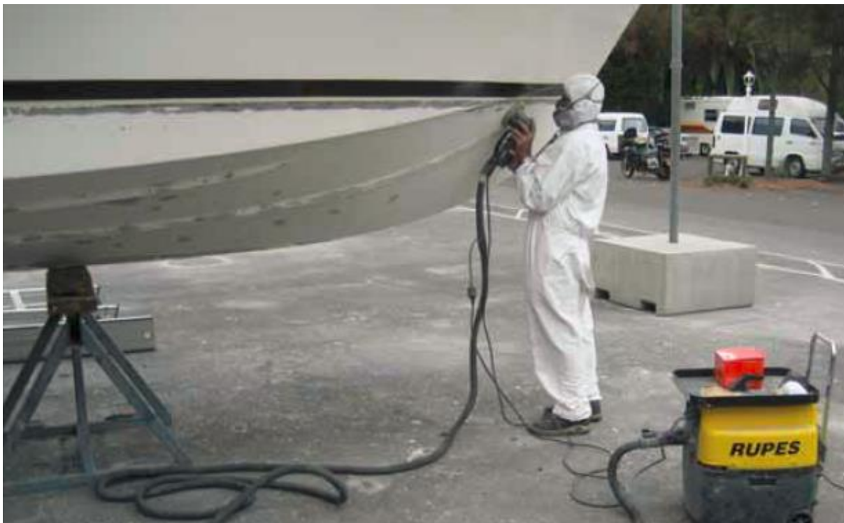
Antifouling removal using a dust collecting sander
