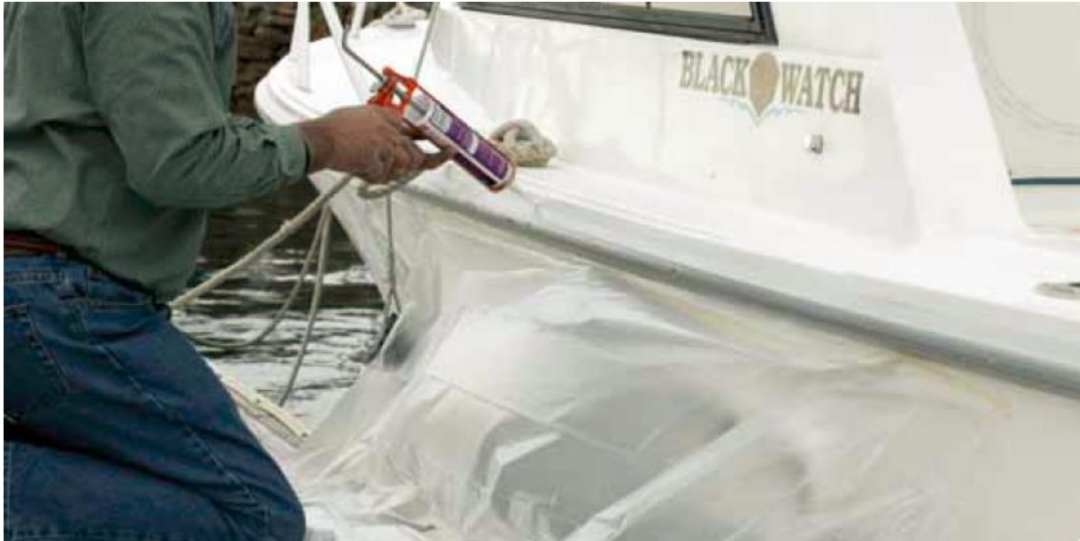
Boat being repaired with masking from the hull to the wharf
