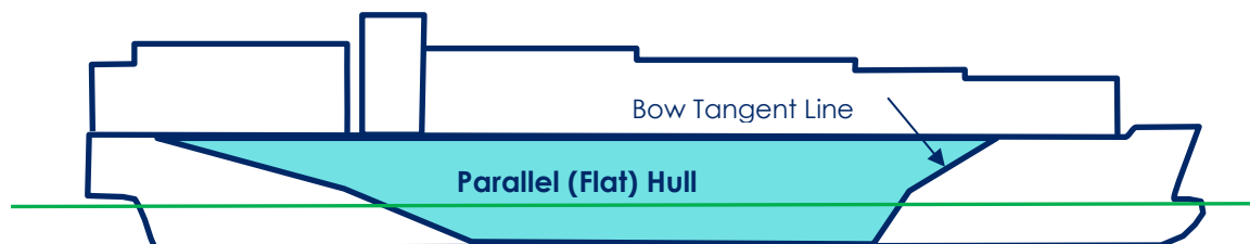
Figure 3.1: Parallel mid-body of a typical container vessel hull
