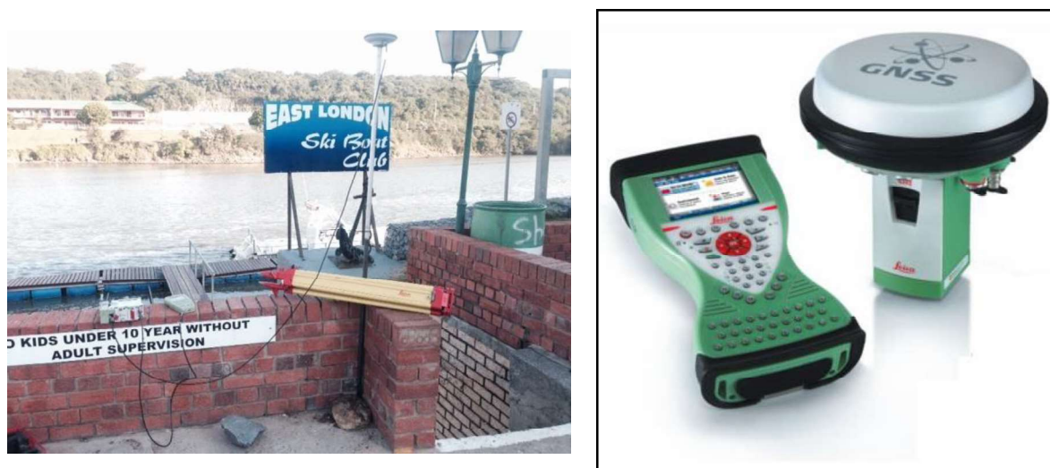
Figure 6: Leica base station (left) and GS15 controller and GNSS GS15 receiver (right).
