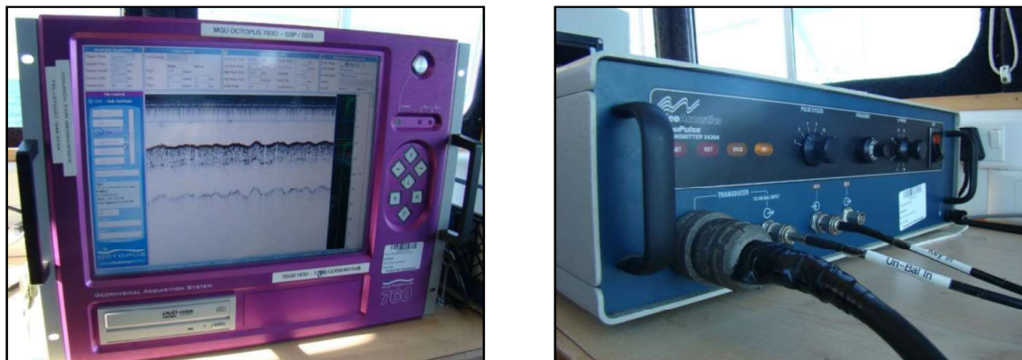
Figure 7. Pinger seismic profiling equipment of Octopus 760D acquisition unit (left) and GeoAcoustics Geopulse transmitter (right).
