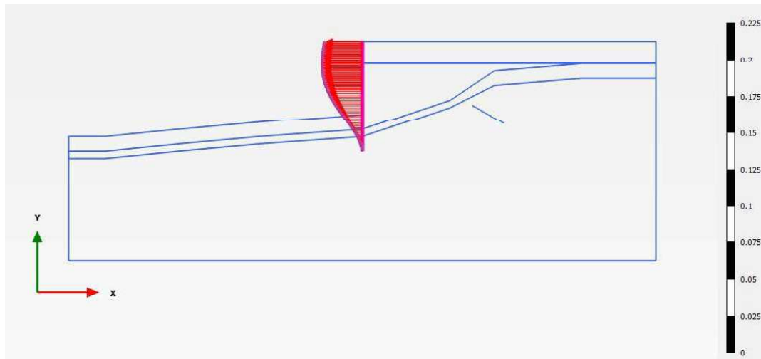
Figure 11: LC5- Horizontal wall displacements
