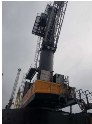
Figure 10(c) MHC 600 sub-components (handrails, catwalks, engine room, winch room, radiator section, boom)
