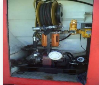
Figure 7(b) Fuel bowser pump arrangement.
