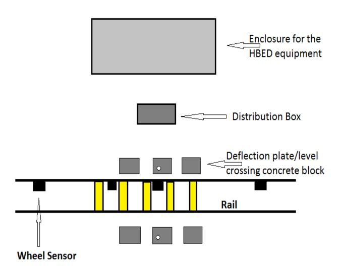
Figure 1 – Typical layout and showing sleepers painted yellow.
