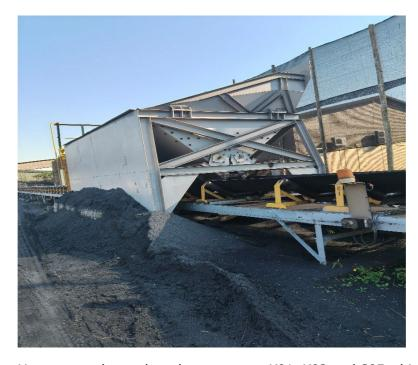
Hoppers are located on the conveyors K01, K03 and S05 which are open stack conveyors where there are cargo stockpiles (Chrome and Magnetite) next to the conveyors. Branded Bakkies must be used to access site.
